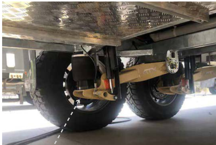
CRUISE MASTER ATX - JACKING POINTS
