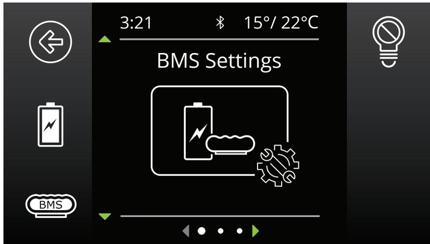
When a Battery Management System is connected, the system will allow setup and modification of a number of BMS settings as outlined below.
