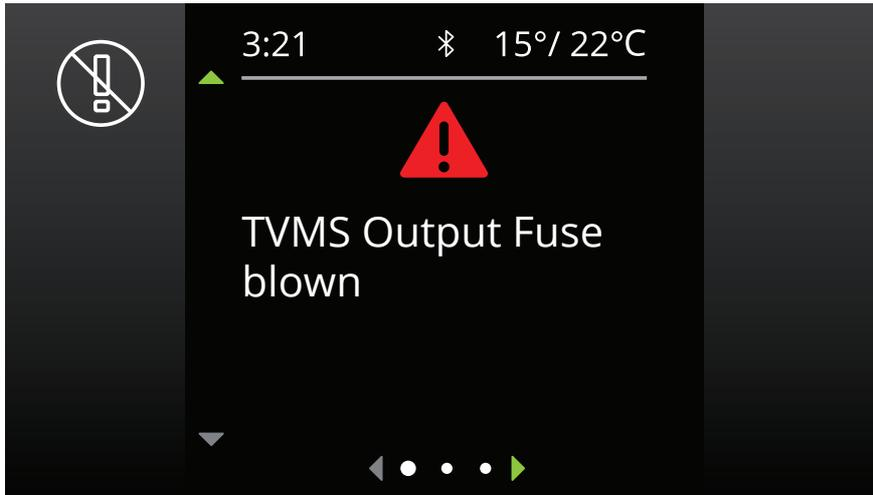
Fault screens will be shown if either an output fuse is blown, the Manager has a fault, or if the unit encounters a switching fault.
