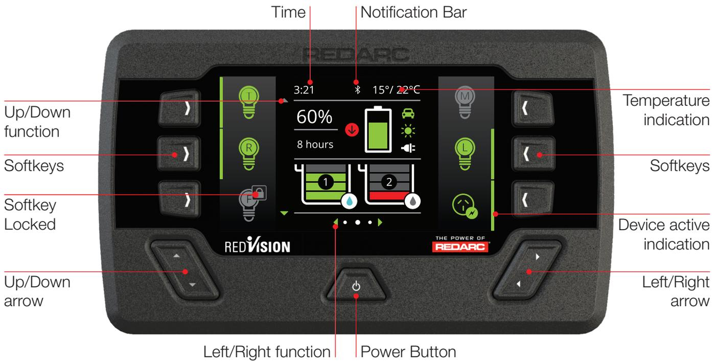
The Display is the main user interface for the RedVision System. It brings information and control to one place without the need for multiple displays and control panels. It is to be mounted in a sheltered location and is the base for control and display for RedVision. It also provides the Bluetooth® interface for the RedVision App.
