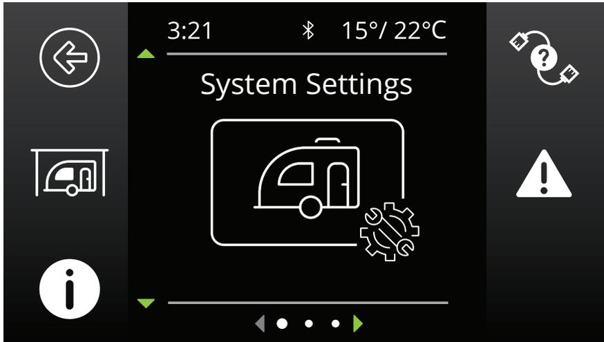
The System Settings screen allows modification of the current operating mode as well as providing information on the system and previous fault history. Each icon is described below.
